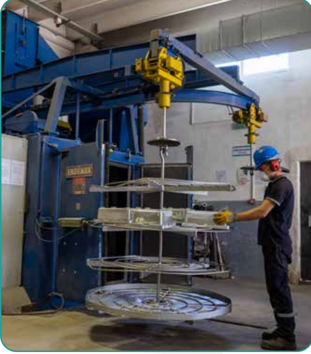
1800x1600 mm 4 Türbinli Kumlama Makinesi 1800x1600 mm 4 Turbine Shot Blasting Machine
