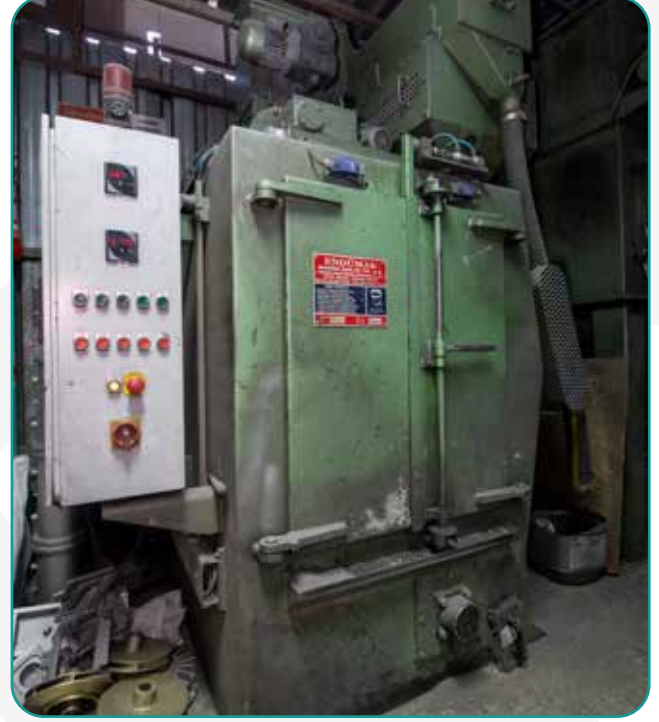
85x100 mm 2 Türbinli Kumlama Makinesi 85x100 mm 2 Turbine Shot Blasting Machine
